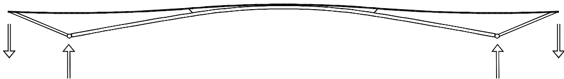
Fig.1 Stress-ribbon stiffened by an arch
