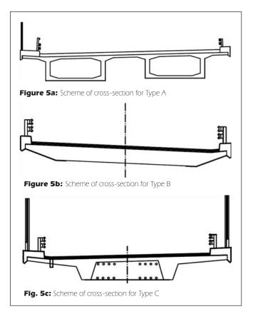
The fundamental difference between the "prototype" bridges is the form of their cross-sections. The selected forms are widely used in practice and represent the majority of girder bridge cross-sections. The ratio of area of the deck slab to that of the whole cross-section is 0.56 for Type A, 1.0 for Type B and 0.64 for Type C.
