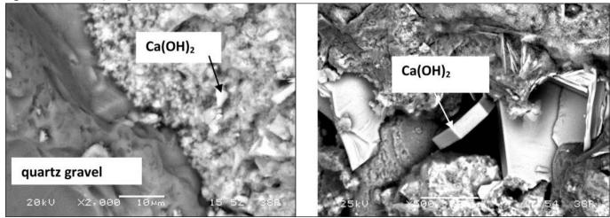
Fig. 25: Concrete with quartz gravel
