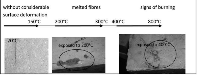
Fig. 13: Concrete specimens with macro fiber reinforced concrete
