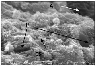
Fig. 7: N 5000 (SEM) Concrete using slag Portland cement Notation: A aggregate quartz gravel, P portlandit, CSH calcium-silikat-hidrat
