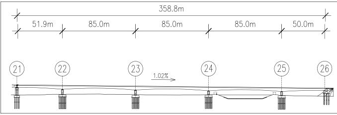
Fig. 3: Side view of the second dilatation unit (DC2)
