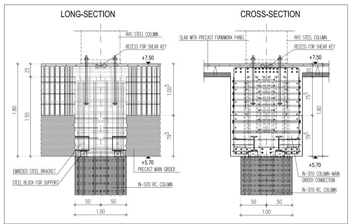
Fig. 6: Connection details of column and main girders
