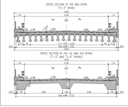
Fig. 17: Cross-section of the Perkáta bridge
