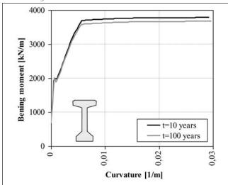
Fig. 7: Bending moment – curvature diagrams of the SHI120-32.80 beam at different ages
