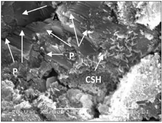
Fig. 6: N 5000 (SEM) Concrete using Portland cement Notation: A aggregate quartz gravel, P portlandit, CSH calcium-silikat-hidrat
