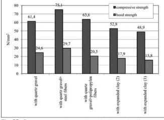
Fig. 23: Concrete compressive strength and bond strength with various mixes at 20  $^\circ\mathrm{C}$
