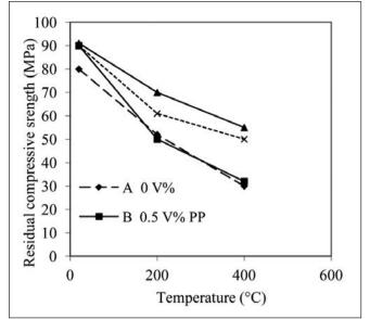
Fig. 19: Residual compressive strength of high strength concrete with or without fibres (Horiguchi, 2005)
