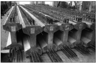
Fig. 11: Manufactured SHI90 beams at Majosháza site
