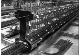
Fig. 10: Reinforcement of the SHI90 beams
