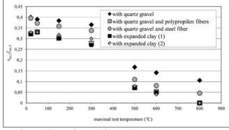
Fig. 24:  $\tau_{_{bu,T}}/f_{_{cm,T}}$  as a function of maximal temperature
