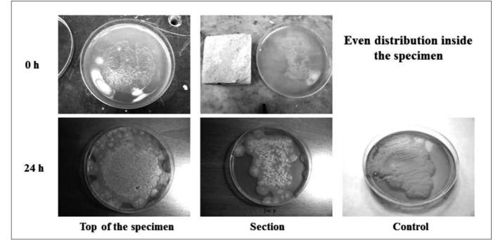
Fig. 6: Indirect evaluation of the effective penetration depth. Prints at 0 h and after 24 hours of incubation, and the control
