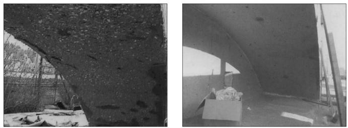
Fig. 17: Tunnel segments after exposure to 1200 °C temperature (Mörth, Haberland, Horvath, Mayer, 2005) a) without fibre reinforcement b) with 2 kg/m<sup>3</sup> polypropylene fibre reinforcement
