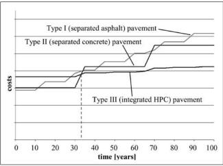
Fig. 7: Calculated life-cycle costs as function of service life for deckpavement superstructures with Type A deck
