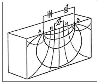
Fig. 1: Theoretical arrangement of direct current measurement
