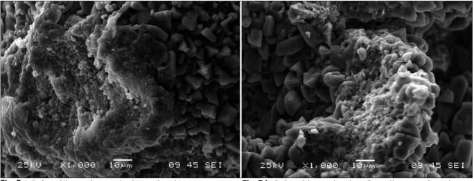
Fig. 5.a: Surface of the sample: original surface on the right, precipitation on the left at 1000 X magnification.
