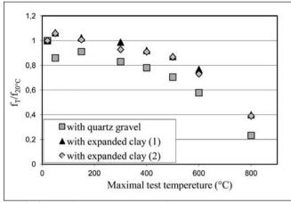
Fig. 8: Change of compressive strength after exposing the concrete to high temperature, measured at room temperature (20°C)
