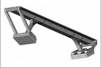
Fig. 12: The model of the M31 bridge in 3D by the Finite element software
