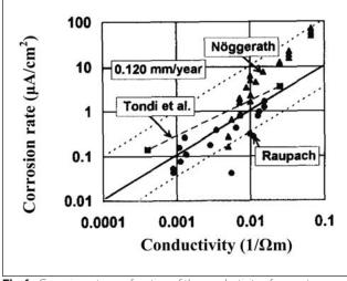
Fig 6: Corrosion rate as a function of the conductivity of concrete or mortar (Hunkeler, 1993)
