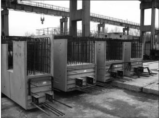
Fig. 8: Precast concrete main girder in the manufacturing yard
