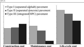
Fig. 6: Calculated costs of deck-pavement superstructures with Type A deck
