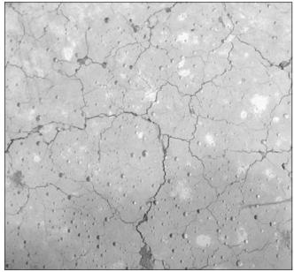
During fire the mechanical characteristics of the concrete are changing. During the cooling process concrete is not able to recover its original characteristics. Deterioration of concrete at high temperatures has two forms: local damage in the material itself (*Fig. 1*) and global damage resulting the failure of the elements (*Fig. 2*). Recent results by Horiguchi (2011) indicated that in some situations a part of the strength can be recovered.
