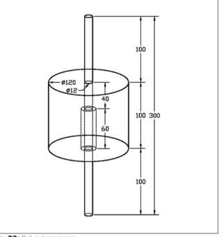
Fig. 22: Pull-out specimen
