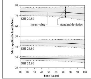
Fig. 8: Change of the mean value and standard deviation of load carrying capacity in case of different SHI120 beams
