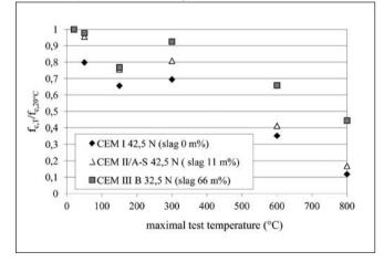
Fig. 4: Compressive strength of hardened cement paste as a function of maximal temperature and cement type
