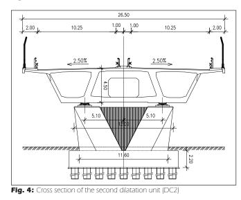
Later, because of constructability, speed of contstruction and financial reasons the design has changed to two dilation units (called DC1 and DC2) with two different types of superstructures, and two totally different methods of construction.
