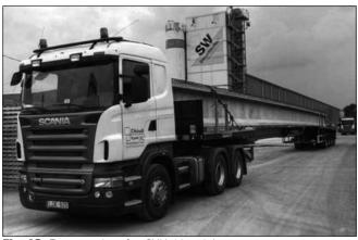
Fig. 13: Transportation of an SHI bridge girder
