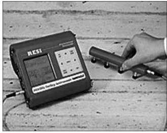
saturated with water preliminarily for electrical conductivity.
