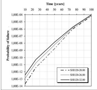
Fig. 9: Change of the probability of failure in case of different SHI120 beams
