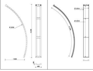
Fig. 6: Plan of the formwork and of the reinforcement for the station of the Fővám-square
