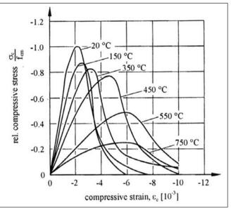
Fig. 3: Stress-strain relationship for concrete with quartz gravel aggregate as a function of temperature (Schneider, Lebeda, 2000)
